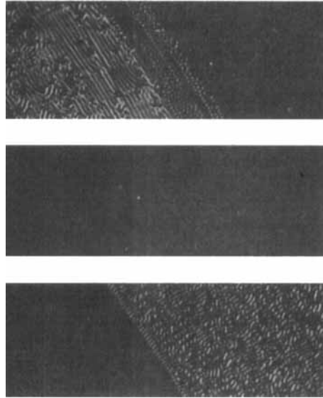
FIGURE 3 Textures of the unipolar response of the nematic film to a DC voltage of -2V (top); 0V (middle) and 2V (bottom).
